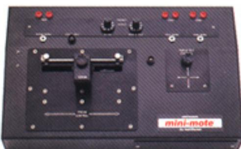
The One Person Video Desk features two non-displacement, pressure sensitive type joysticks. A dual axis type for pan and tilt, and a single axis type for zoom. A linear (L-R) slider controls focus.
