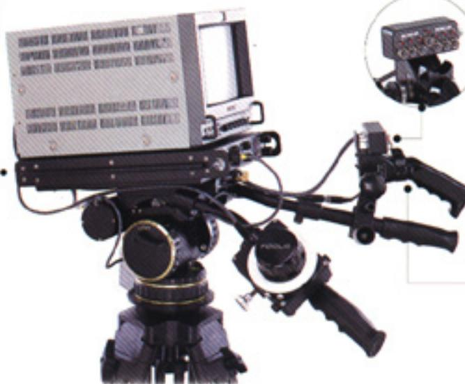
The Divide-By/Multiply-By feature allows the operator to increase or decrease his pan and tilt movement by factors of 2x, 4x or 8x. The center reset button allows instantaneous resumption of 1:1 head control.
